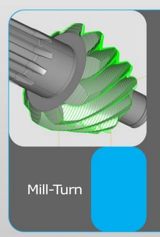
OneCNC Mill-Turn added module software gives you the tools and simulation to provide a logical visual method of programming your mill-turn lathes. OneCNC Mill-Turn simplifies even the most complicated parts by providing wizard driven active plane access to all required faces of the mill-turn part.
